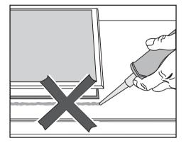
The sealing strip under the edge of the top part of the appliance provides a sufficient seal for the worktop.
